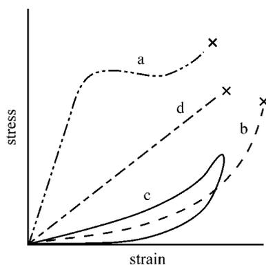
**Figure 2.** Shape comparison of stress–strain curves. a) The general S-shaped curve of artificial materials. b) The J-shaped curve of 3DFs, soft biological tissues (such as skin and muscle) and fibrocartilaginous tissues. c) Hysteresis-loss curve for biological materials. d) The linear elasticity of artificial materials that obey Hooke's law and Newton's law. X is the break point.
