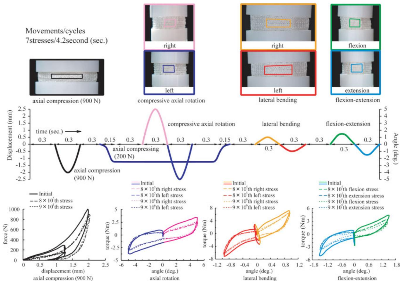
**Figure 4.** Change in hysteresis loss and the maintenance of dynamic motion in a 3DF disc during a simulated 30 year in vivo period under harsh, dry conditions. The 3-DF disc kept the same profiles as those for 10 and 20 year in-vivo periods. The strain change in each hysteresis-loss curve in response to a given stress is shown as a component of the total cyclical motion that accompanies each distortion of 3DF disc.
